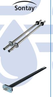
Multi Point Air velocity Probes The AV-EP series of air velocity probes are available in lengths from 100 to 600mm and the AV-MPS series in lengths of 700 to 2000mm. They are used to ensure that recommended flow rates for public buildings and industrial plants are achieved. They can be connected to a PA-60x, PA-65x, PA-699 Air Differential Pressure Sensor of an appropriate range.
