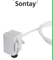
**True Duct Averaging Sensors**The TT-626 true duct averaging sensor contains a PT100b element, which measures at every instantaneous point along the full length of the 10mm diameter copper tube and is suitable for use in the range -30 to +70°C
